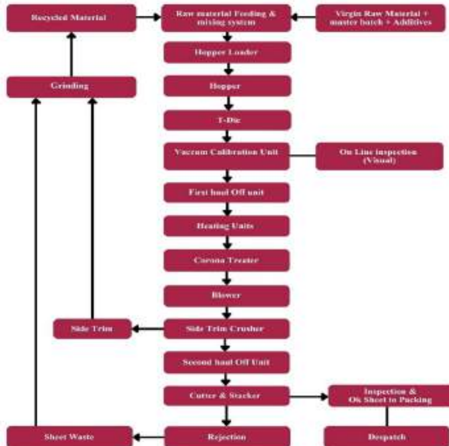
Flow Chart of the Extrusion Process. (PP Flute Boards)
